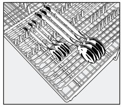
Spoon heads should be placed in contact with the serrated retainers of the cutlery tray so water can run off.
